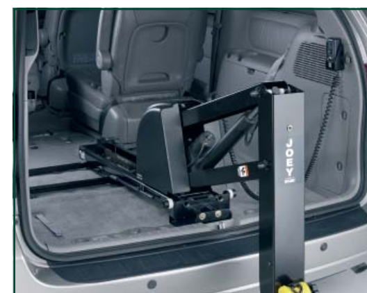
The compact rail design uses only the third row seat fixings in the floor.
