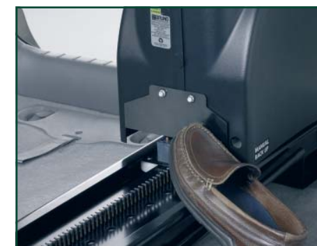
Safety plate obstruction sensor.
