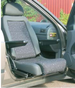
The Turnout swivel base turns the chair outwards, so Carony Go can be docked to the car.
